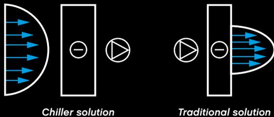
in the noise levels it produces. When the coil is fitted on the intake side of the fan (see image), the air profile remains at a steady level. In contrast, when the coil is on the pressure side of the fan, the air goes directly through the coil, requiring an increase in the air flow in order to attain the desired cooling output.
